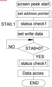
Note: this command is available when hardware column number and software column number are the same. Hardware column number is related to MD2 and MD3 setting. Software column number is related to ser text area and set graphic area command.
