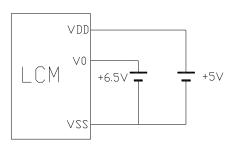
V<sub>DD-</sub>V<sub>0</sub>: LCD Driving voltage VR: 10k~20k
