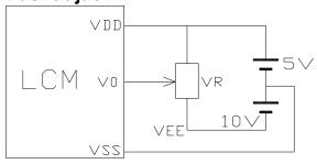
VDD~V0: LCD Driving voltage
