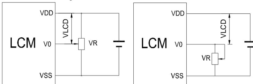
V<sub>DD</sub>-V<sub>0</sub>: LCD Driving voltage
