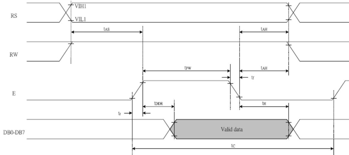
**Write cycle** (Ta=25°C, VDD=2.7V)
