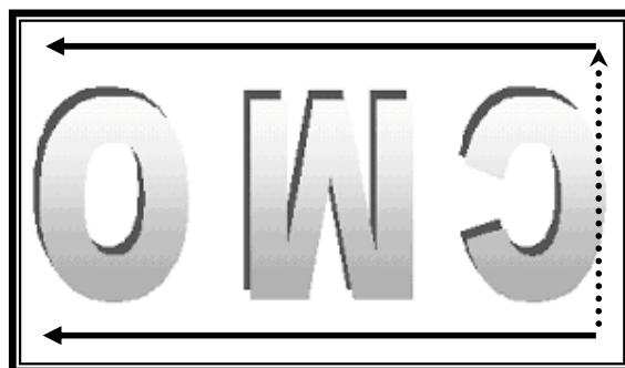
RPF1 = high: display with 180degree rotation
