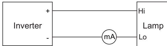
(Figure. 1: Measurement of return current)
