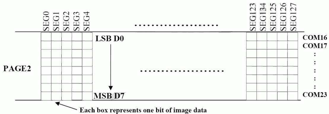
Enlargement of GDDRAM (No row re-mapping and column-remapping)
