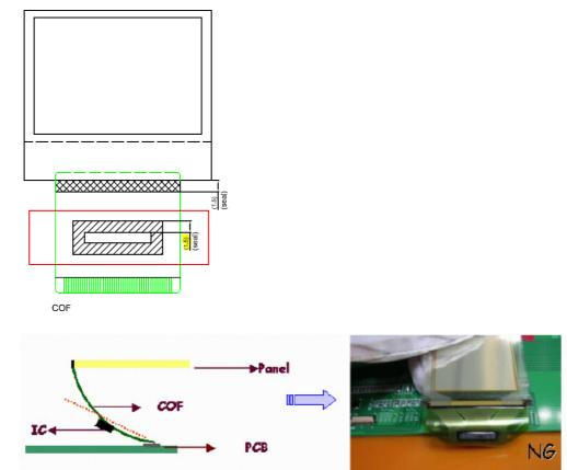
10. Use both thumbs to insert COF into the connector when assembling the panel. Please refer to the photo.
