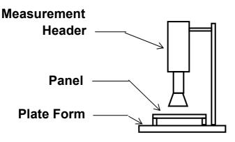
PR-670 / MINOLTA CS-100 Color Analyzer
