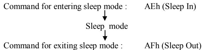
**Figure 8-17 : Case 2 - Command sequence for disabling internal V<sub>DD</sub> regulator during sleep mode**
