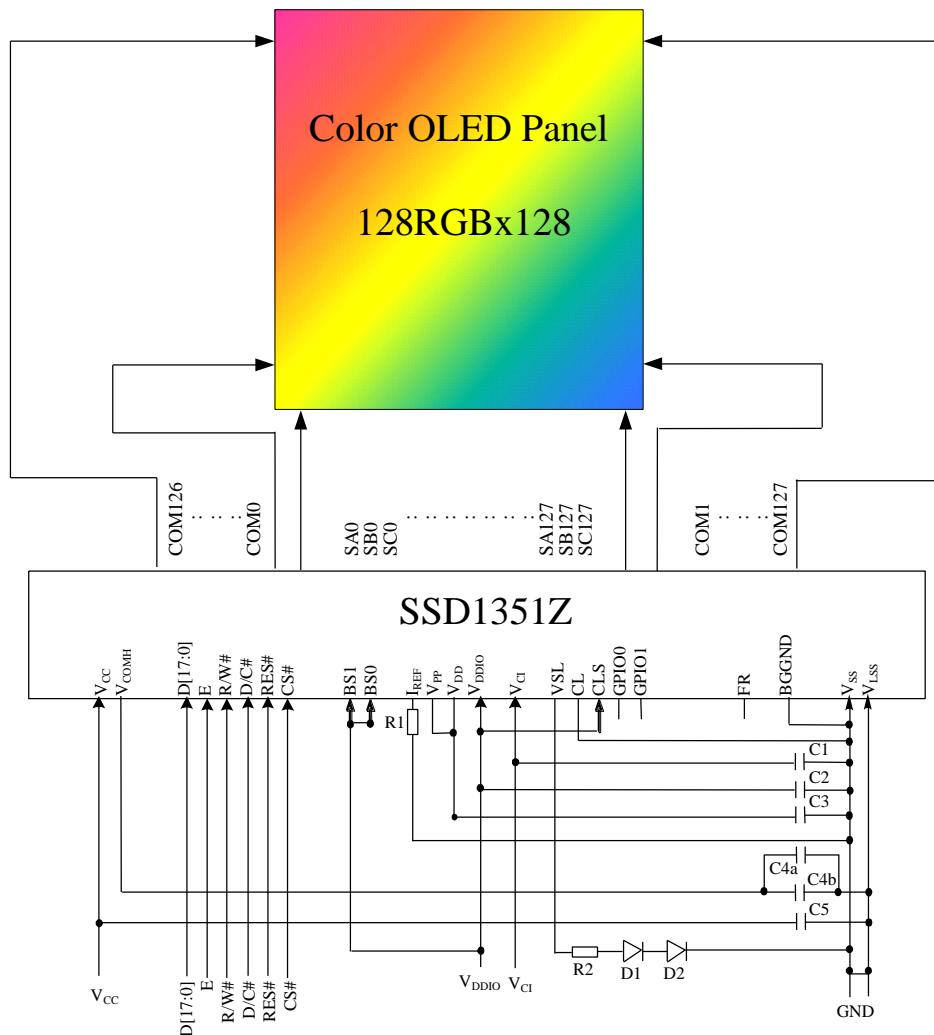
Voltage at  $I_{REF} = V_{CC} - 6V$ . For  $V_{CC} = 16V, I_{REF} = 12.5\mu A$ :
