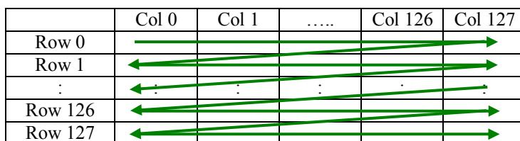
When A[0] is set to 1, the driver is set to vertical address increment mode. After the display RAM is read / written, the row address pointer is increased automatically by 1. If the row address pointer reaches the row end address, the row address pointer is reset to row start address and column address pointer is increased by 1. The sequence of movement of the row and column address point for vertical address increment mode is shown in Figure 10-3.
