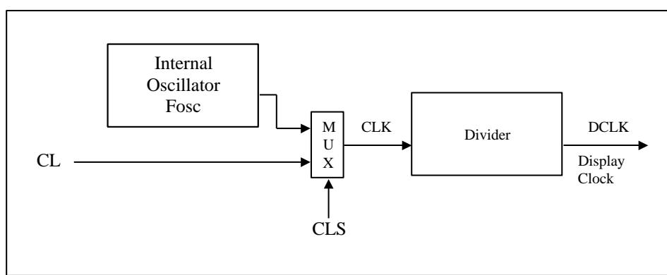
This module is an On-Chip low power RC oscillator circuitry (Figure 8-7). The operation clock (CLK) can be generated either from internal oscillator or external source CL pin by CLS pin. If CLS pin is HIGH, internal oscillator is selected. If CLS pin is LOW, external clock from CL pin will be used for CLK. The frequency of internal oscillator  $F_{osc}$  can be programmed by command B3h.
