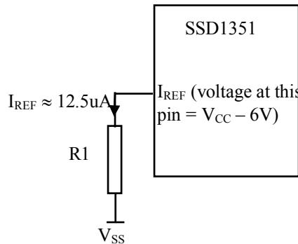
Since the voltage at  $I_{REF}$  pin is  $V_{CC} - 6V$ , the value of resistor R1 can be found as below:
