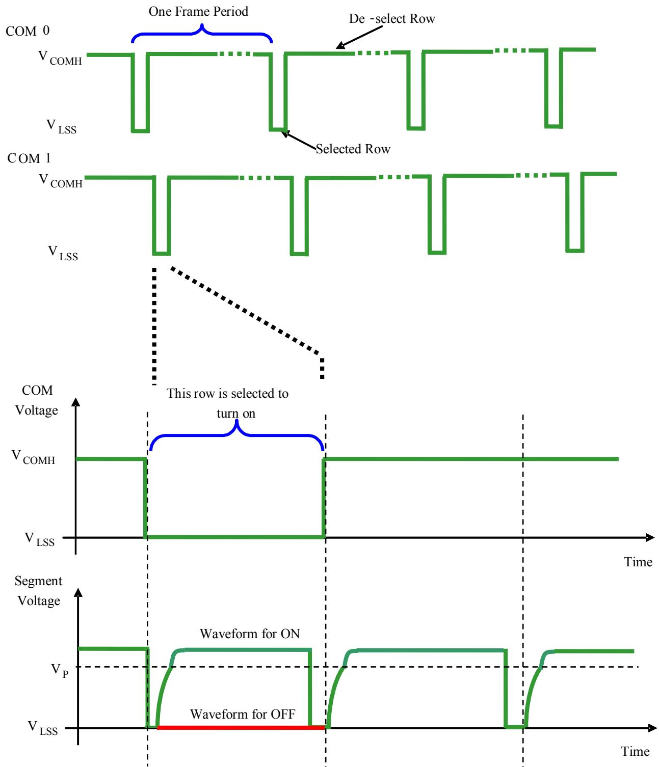
There are four phases to driving an OLED a pixel. In phase 1, the pixel is reset by the segment driver to  $V_{LSS}$  in order to discharge the previous data charge stored in the parasitic capacitance along the segment electrode. The period of phase 1 can be programmed by command B1h A[3:0]. An OLED panel with larger capacitance requires a longer period for discharging.
