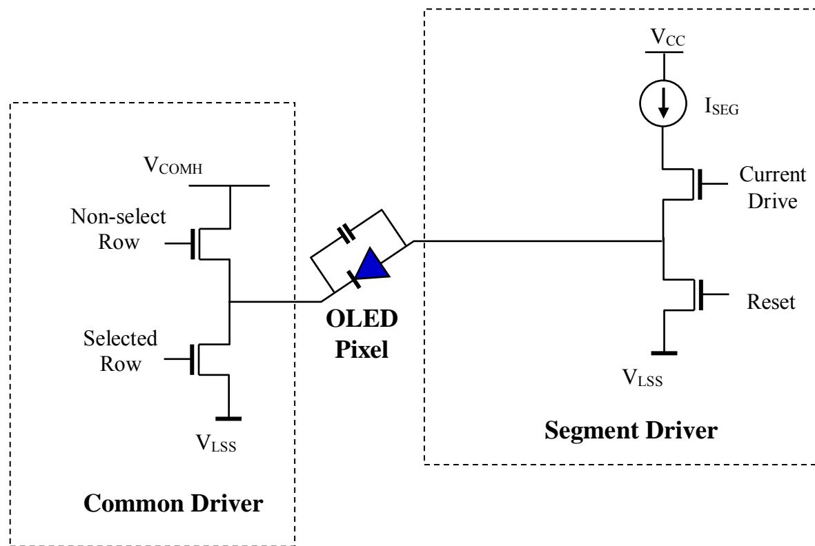
The commons are scanned sequentially, row by row. If a row is not selected, all the pixels on the row are in reverse bias by driving those commons to voltage  $V_{COMH}$  as shown in Figure 8-10.
