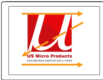
Fig. 1 Normal scan (Pin19, RSV = Low or NC)
