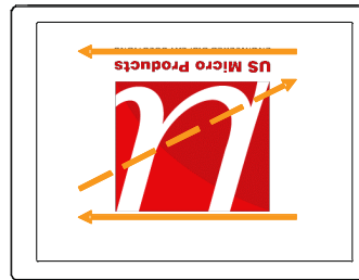
Fig. 2 Reverse scan (Pin19, RSV = High or VDD)
