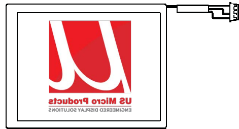
Fig. 2 Reverse scan (DPSH = Low/NC, DPSV=Low)
