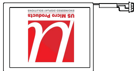
Fig. 4 Reverse scan (DPSH = Low, DPSV=High)
