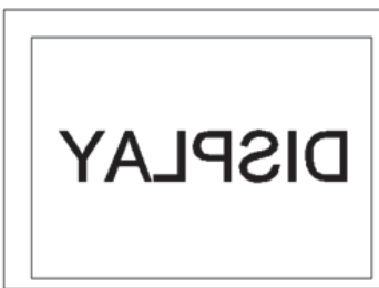
Fig. 9.10 Horizontal reverse (U/D: High; L/R: Low)
