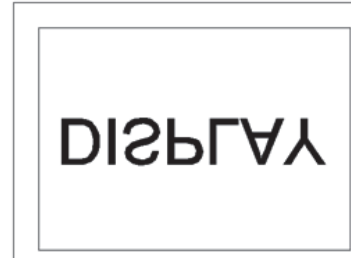
Fig. 9.9 Vertical reverse (U/D: Low; L/R: High)
