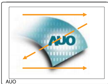
Fig. 1 Normal scan (Pin4, REV = Low or NC)
