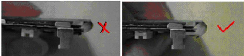
9. Avoid bending the film at IC bonding area. It could damage the IC ILB bonding. It should avoid bending the IC seal area. Please keep the bending distance >1.5mm.
