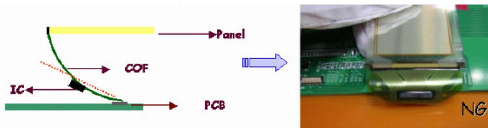
10. Use both thumbs to insert COF into the connector when assembling the panel. Please refer to the photo.
