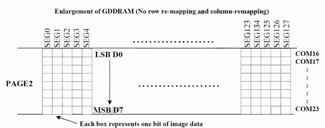
For mechanical flexibility, re-mapping on both Segment and Common outputs can be selected by software.
